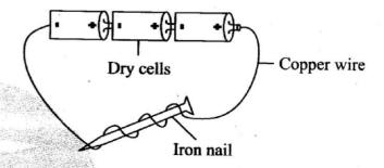
The correct energy transformation for the above electromagnet is
