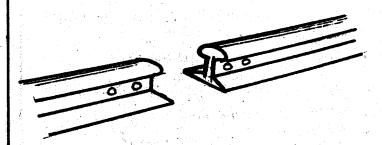
Small gaps are left between the railway lines in order to:-
