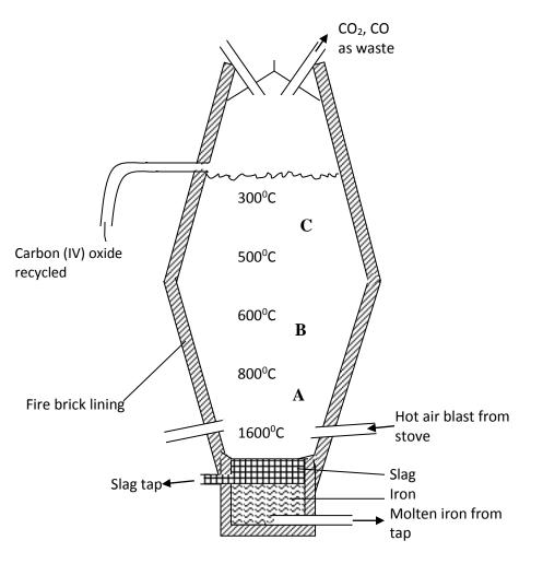
(a) (i) What does the word smelt mean? (1 mark) *Extraction of a metal from its ore using a reducing agent and heat.*
