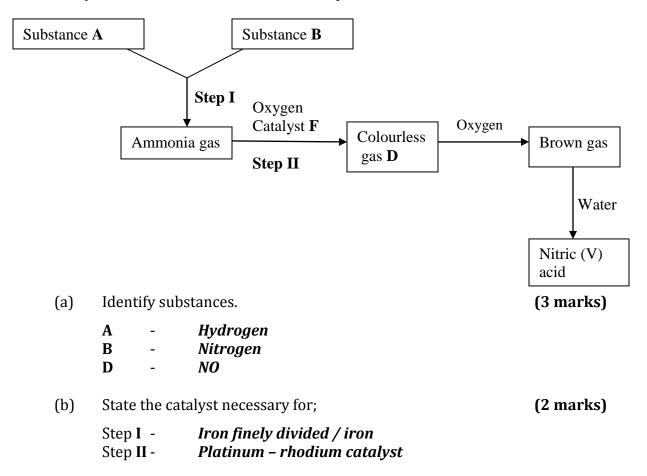
(c) Write a balanced chemical equation for taking place in step **II**. **(1 mark)**
