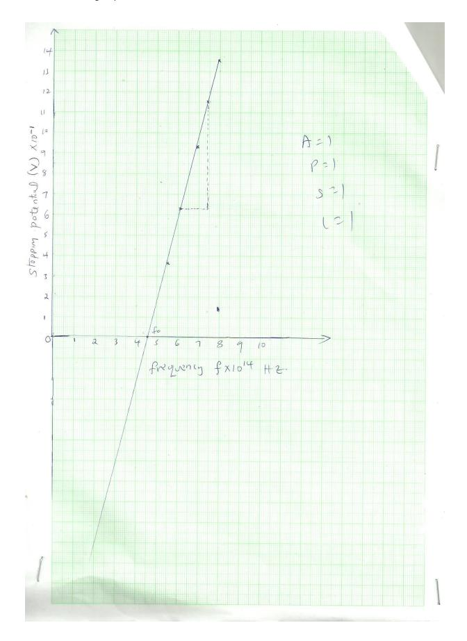
iii) Determine plank's constant, h and the work function of the surface given that  $eV_s = hf - hf_o$ , where  $e = 1.6 \times 10^{-19} \, C$  (3mks)
