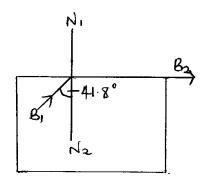
B2 is the emergent ray of B1. Determine the refractive index of the glass block.
