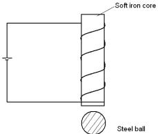
In order to lift a slightly heavier ball, it is necessary to make a stronger electromagnet. State two ways in which the electromagnet could be made to lift a heavier steel ball. (2 marks)
