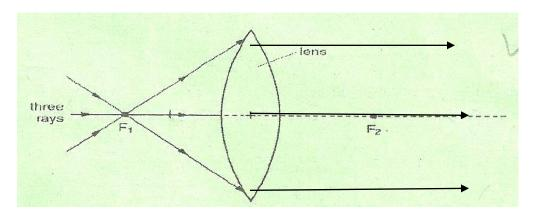
Three rays of light pass through F<sub>1</sub> to the lens.
