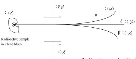
Working diagram,  $\alpha$  should be deflected less than  $\beta$  because of its heavier mass.
