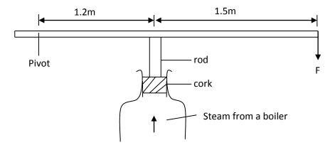
If the area of the cork is 15 cm<sup>2</sup> and a force (F) of 500N is needed to keep the cork in place, determine the pressure of the steam in the boiler. (3mks)
