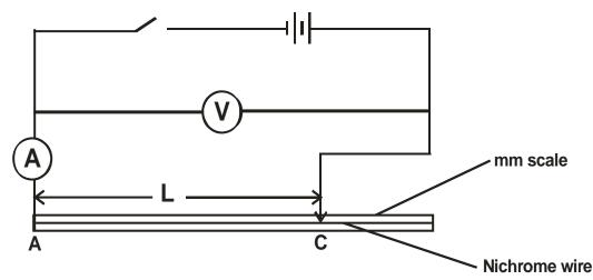
b) Connect the ends A and C where AC is the length L of the Nichrome wire across the terminals as shown. Close the switch and measure both current I and potential difference (P.d) across the wire AC when L = 100cm.
