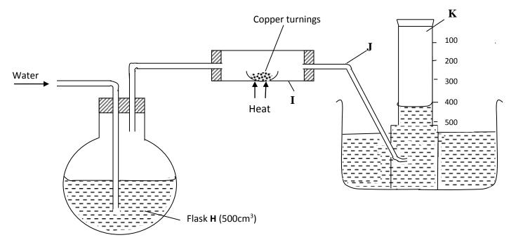
A  $500 \text{cm}^3$  measuring cylinder **K** was filled with water and assembled for gas collection. Copper turnings were heated red hot and water was slowly passed into  $500 \text{cm}^3$  flask **H** until it reached the  $500 \text{cm}^3$  mark. A colourless gas was collected in **K**.
