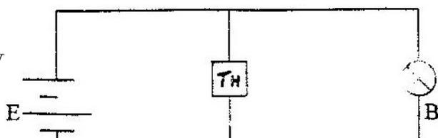
Thermistor, TH, is connected in parallel with a bulb as shown in figure 3. The bulb is lit. When the thermistor is steadily heated the brightness of the bulb reduces. Explain this observation
