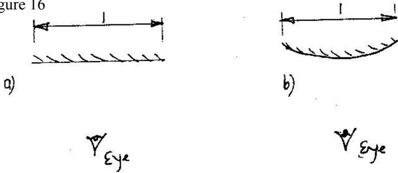
By sketching a pair of incident and reflected rays for each (a) and (b) show how the convex mirror provides to the eye, a wider field of view than the plane mirror.
