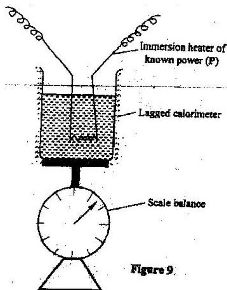
Describe an experiment to determine the specific latent heat of steam,  $l$ , using the set up. In your answer clearly explain the measurements to be made and how these measurements could be used to determine  $l$ . (6mks)
