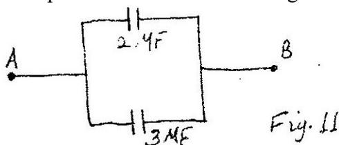
Determine the p.d across AB given that the total charge in the capacitors is  $1 \times 10^{-4}$  Coulombs.
