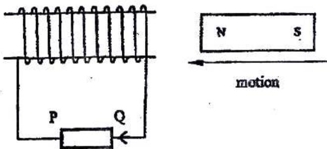
10. Figure 5 shows a magnet being moved towards a stationary solenoid. It is observed that
