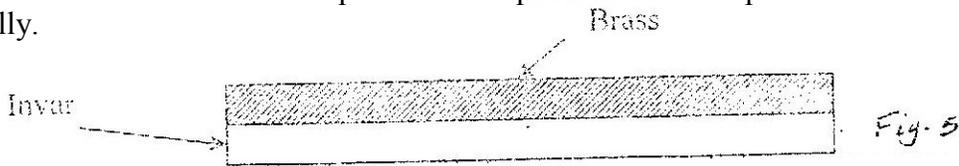
Sketch the bimetallic strip after being cooled several degrees below room temperature.
