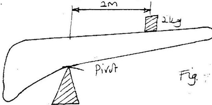
Determine the distance of the center of gravity of the log from the pivot.
