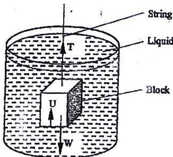
liquid. The three forces acting on block are the tension  $T$ , On the the weight  $W$ , of the block and upthrust,  $U$  due to the liquid.
