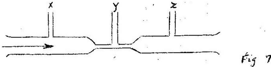
Show on the diagram the relative positions of the levels of the liquid in section marked x, y and z
