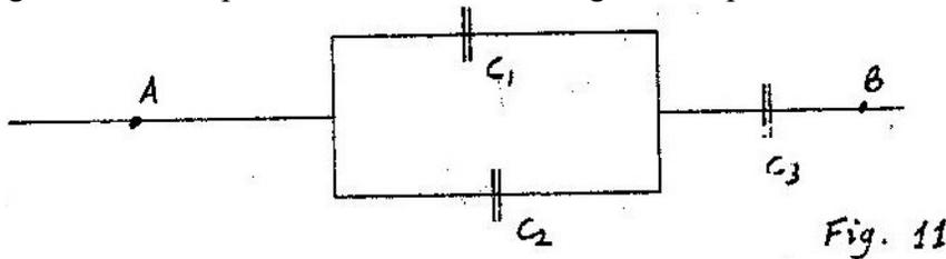
Write an expression for  $C_T$  the effective capacitance between A and B.
