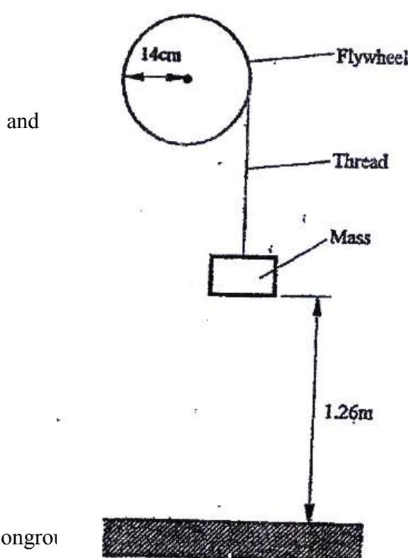
centre so that it can rotate freely about the axis. A thread is wrapped round the wheel and a mass attached to its loose end so as to hang at a point 1.26 m above the ground.
