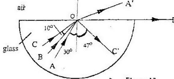
Determine the critical angles of the glass material. **Figure 13**
