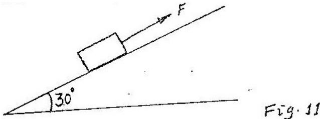
If the distance moves along the incline is 4.0m, determine work done by the force F.
