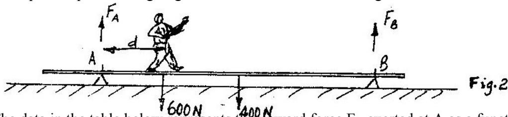
The data in the table below represents the upward force  $F_A$  exerted at A as a function of distance,  $d$ . The distance  $d$  is measured from A.
