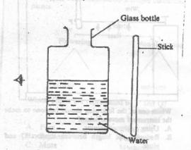
The part of the stick below the level of water appeared to be larger in size than the part above the level of water because rays of light were
