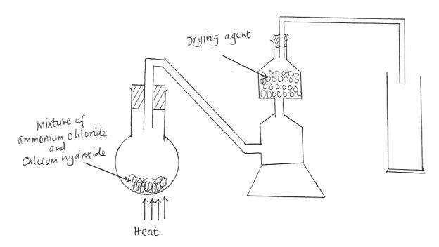
a) Identify two mistakes in the set up and give a reason for each mistake. (2 marks)
