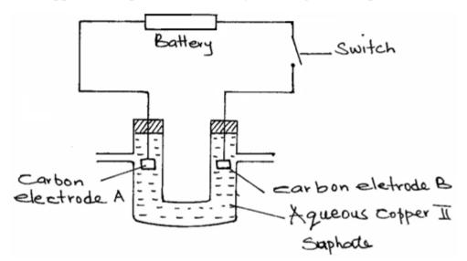
Chemistry Paper 28Cekenas Joint Mock(i)When the switch was closed, a gas was produced at electrode **B**.Which electrode is the anode?
